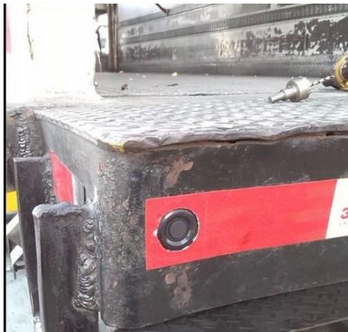
Insert into bumper, then install another shim
