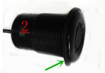
Install the first shim
